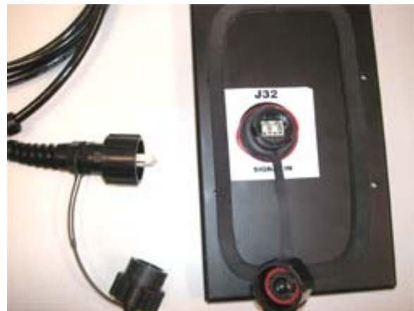
Figure 23: Fiber Interconnect Cable and Input
