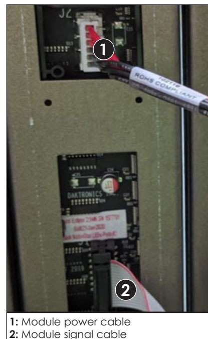
Figure 4: Disconnect Power & Signal Cables from Each Module
