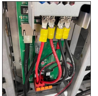
Figure 6: Disconnect Cables from RJ45 Jacks & Power Supply
