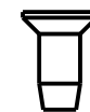
TAP SCR, M5 X 0.8 X 12MM, FLAT HEAD, T25, BLK ZINC PN: HC-4782939 (BORDER HARDWARE & MOD Z-ADJUST HARDWARE)
