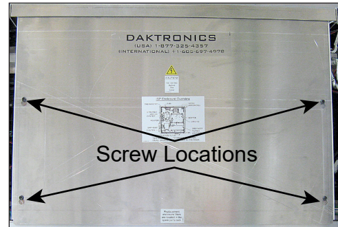
Figure 36: Control Equipment Door
