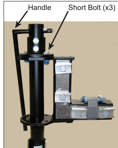
Figure 38: Webcam Arm Bolts
