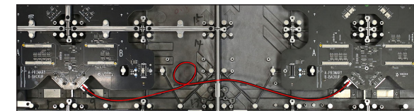
Figure 9: Redundant Horizontal Signal Connection
