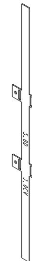
EMI SHIELD BRACKET: USED IN ALL HALF-PANEL FACET DISPLAYS USED IN CONVEX FULL-PANEL FACET DISPLAYS NOT USED IN CONCAVE FULL-PANEL FACET DISPLAYS
