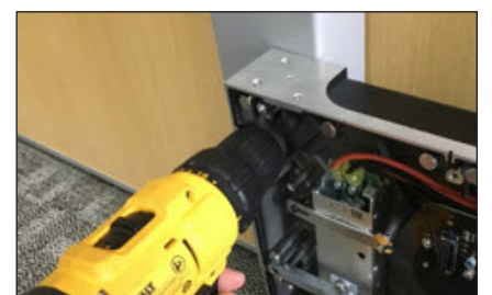
Figure 21: Secure Panel to Tube
