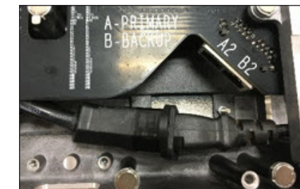
Figure 20: Install Power Input Cable
