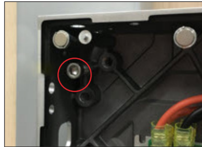
Figure 23: Adjust Jacking Hardware
