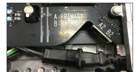
Figure 21: Install Power Input Cable
