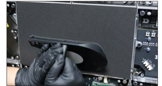
Figure 24: Using Magnetic Removal Tool
