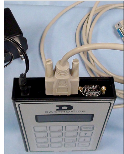
Figure 15: DM-100 Handheld Console Connected for GS6 Display Control
