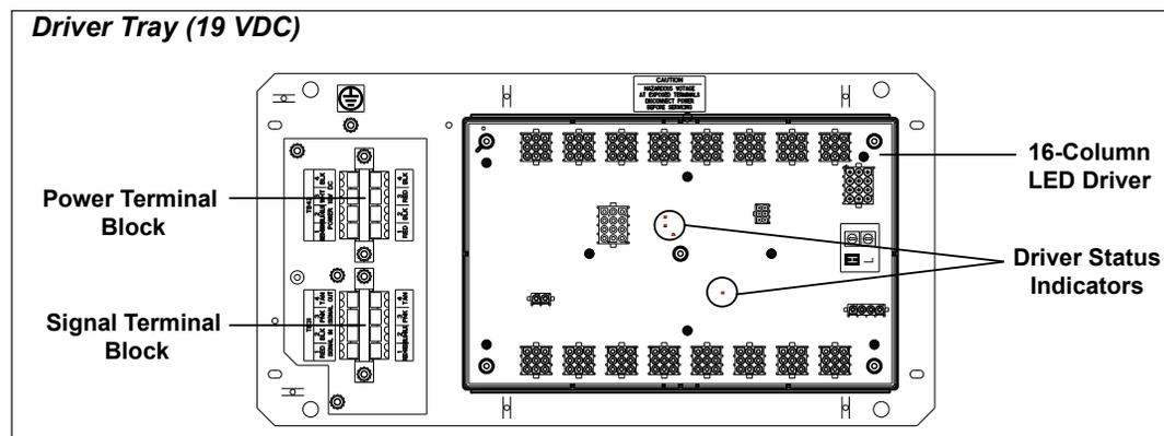
**Figure 9:** 16-Column Driver Tray Components (19 VDC)
