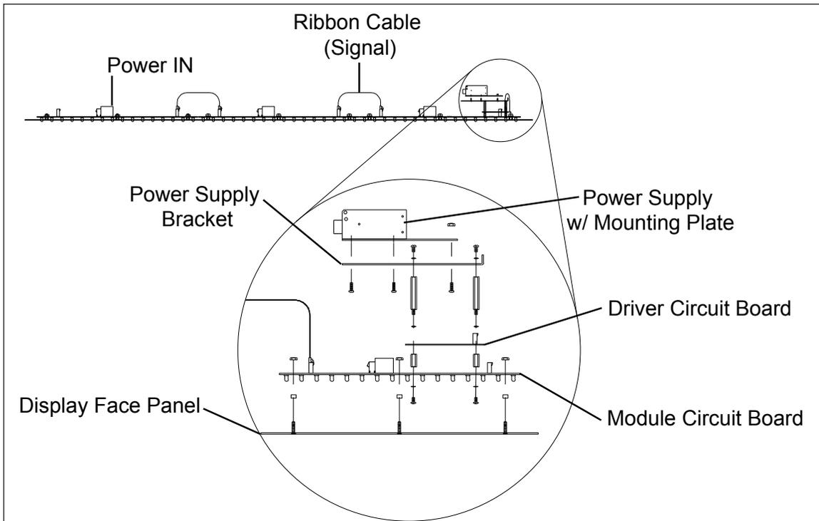
Figure 17: Display Assembly, Top View
