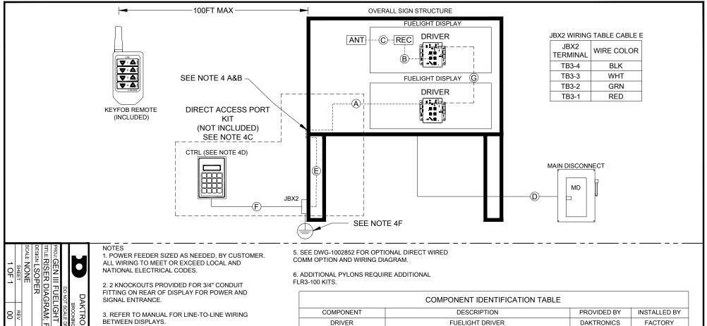
1. POWER FEEDER SIZED AS NEEDED, BY CUSTOMER. ALL WIRING TO MEET OR EXCEED LOCAL AND NATIONAL ELECTRICAL CODES.
