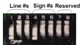
Figure 8: DIP Switches with #1 and #4 ON (pressed down)
