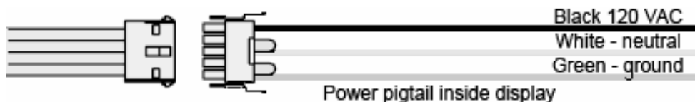
Figure 6: Power Pigtail Wiring
