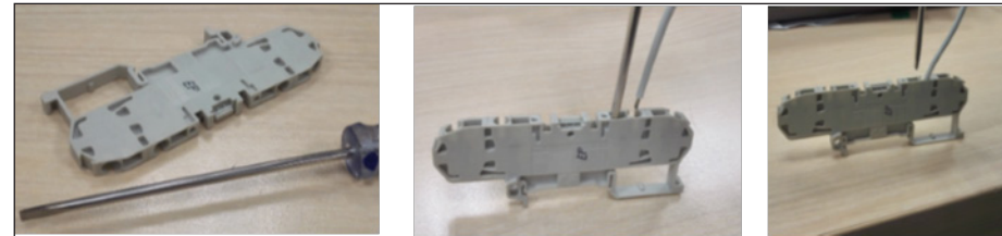
Figure 24: Term Block Installation
