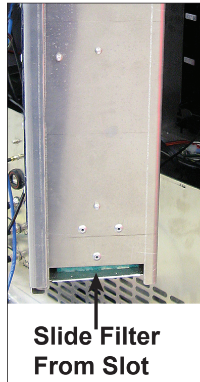
Figure 35: ISP Enclosure Filter Location
