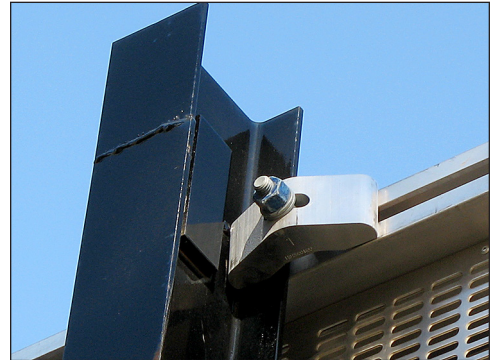
Figure 6: Rocker Clamp Engaging Upright
