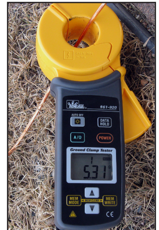
Figure 8: Measure Resistance to Ground
