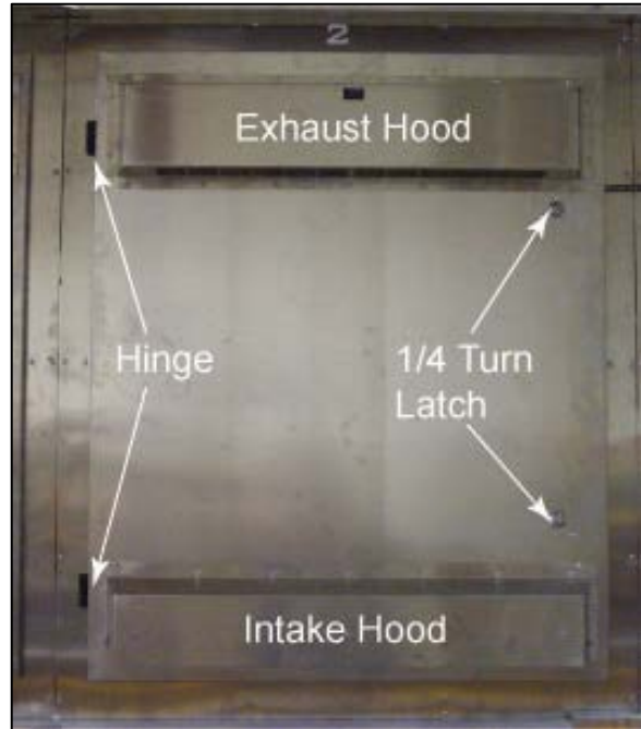
Figure 7: Rear Access Door with Vent Hoods
