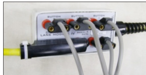
Figure 11: Lane Module with All Connections (Except RTOP)
