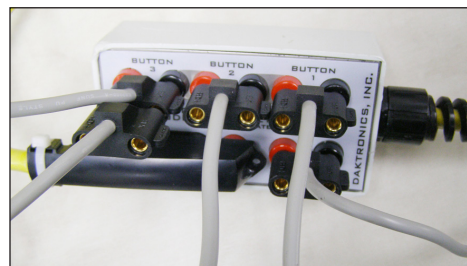
Figure 12: RTOP Connected to BUTTON 3
