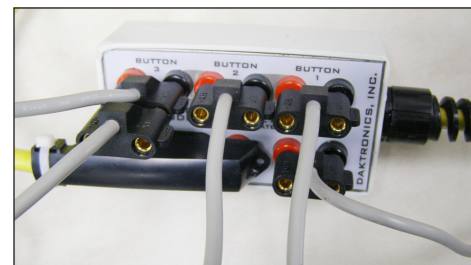
Figure 58: RTOP Connected to BUTTON 3
