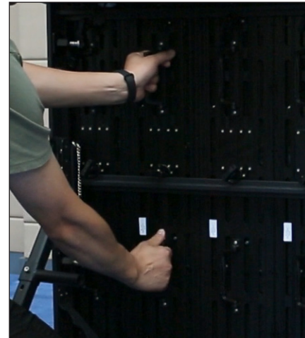
Figure 32: Grasp Handles on Rear of Module
