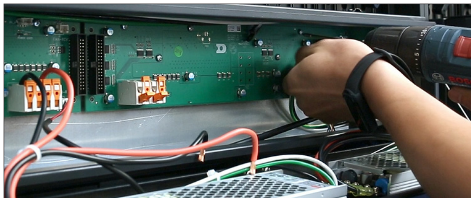
Figure 42: Remove Screws Securing Hub Board to Power Box
