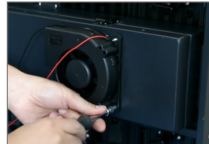
Figure 45: Remove Screws Securing Fan to Power Box
