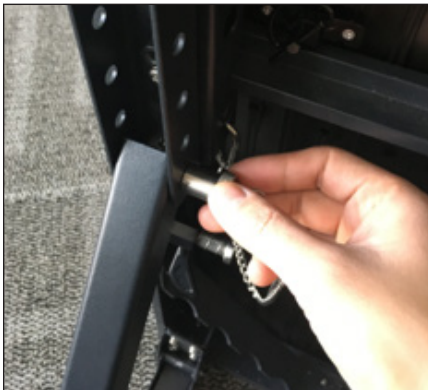
Figure 18: Remove Locking Pin from Stiffener
