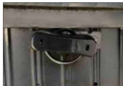
Figure 31: Unlocked Module Latch Position
