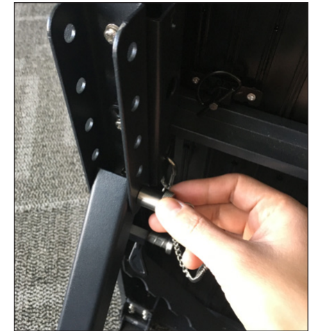
Figure 15: Adjust Angle of Panel
