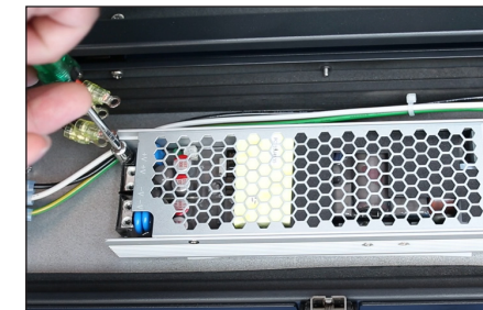
Figure 49: Remove Nuts from Power Supply
