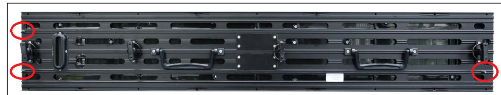
Figure 34: Connector & Locator Pins on Module Rear
