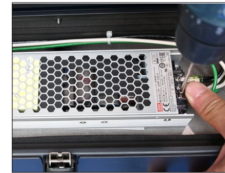
Figure 47: Remove Cables from Power Supply
