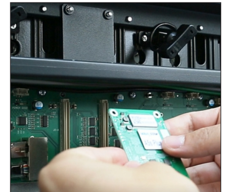
Figure 37: Remove Receiver Card from Hub Board
