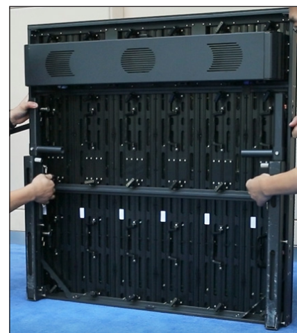
Figure 11: Remove Locking Pins
