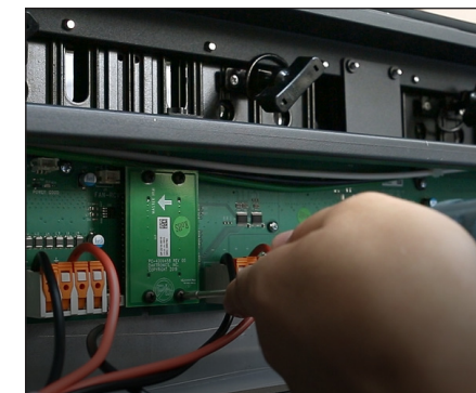
Figure 39: Remove Screws Securing Jumper Board to Hub Board
