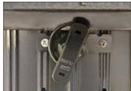
Figure 30: Fully Locked Module Latch Position
