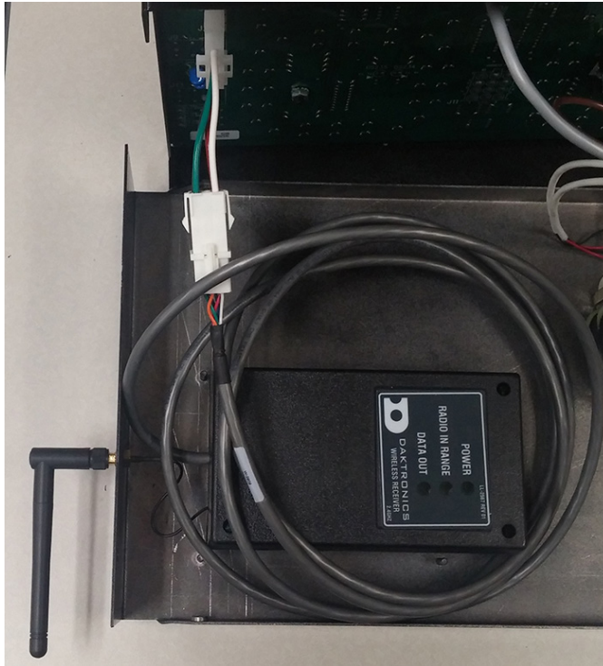
Figure 8: Radio Receiver Installed
